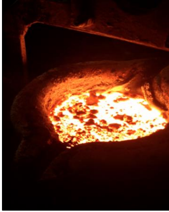
Figure 3.5 Ladle dross formed after magnesium treatment and inoculation.
