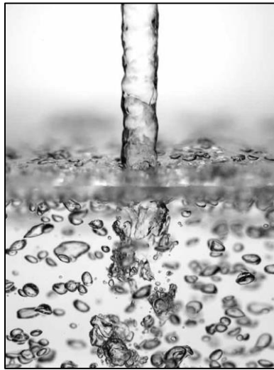
Figure 1.2 Air bubbles near a plunging liquid water jet by “Jesse Belden (NUWC) and Tadd T. Truscott (BYU)” [3].
